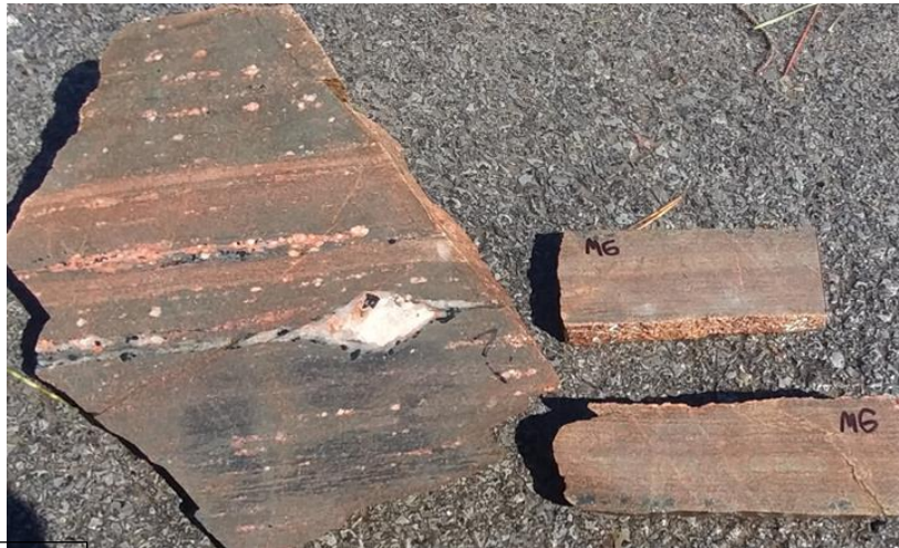
Figure 22. Photograph of the sawn surface of the Median Gneiss sample from Talcville. Note the compositional layering, deformed leucosomal layers, and pink, feldspar porphyroclasts. Black crystals are tourmaline.
