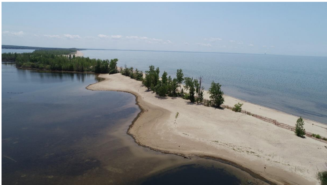
Figure 9. Aerial view of beach nourishment project, north spit of Sandy Pond, Summer 2021. Here, sand dredged from the channel (background, far left) and placed along the shorelines (in front of dune fencing) and
