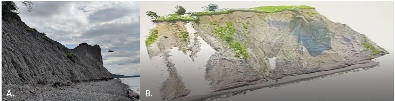
Figure 4: A) Flying the Mavic UAV along the shoreline, collecting imagery of the bluffs B) An example of a 3D model of McIntyre's Bluff created using UAV imagery. The prominent cliff seen in A can also be seen in B. The 3D model was created using Agisoft Metashape software. Models such as this one can be directly compared with others from other time periods, and a percent change in the surface can be estimated.
